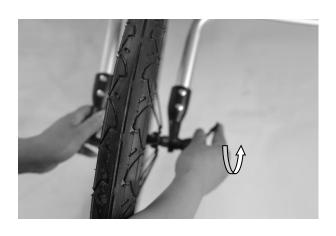
Install the front wheel in the direction shown on the front fork.
