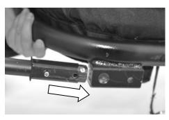
4. Install tow bar into square tube and lock safety pin..
