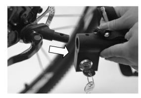
6. Install steel connector onto bike axle. 7.Insert steel connector into the hole(see picture)
